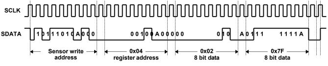
Figure 2. I<sup>2</sup>C Write to Column Size Register (0x04) with the Value 0x027F
