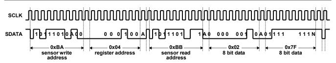
Figure 3. I<sup>2</sup>C Read from Column Size Register (0x04). 0x027F Returned
