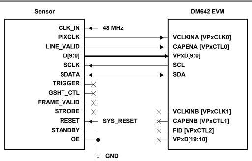
NOTE: /SYS RESET is connected to the RESET switch on the DM642 EVM.
