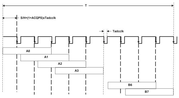
Figure 7. Timing Details of 16 Channel Conversion
