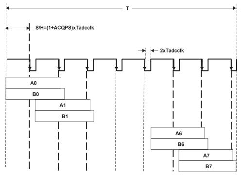
Figure 9. Timing Details of 8 Pairs of Channels
