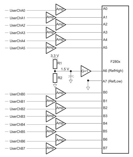
Figure 5. Channels for Calibration, 14 User Channels
