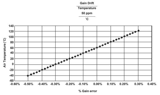
Figure 11. Gain Drift Over Temperature
