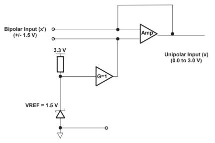
Figure 2. Simplified Circuit for Ideal ADC Case
