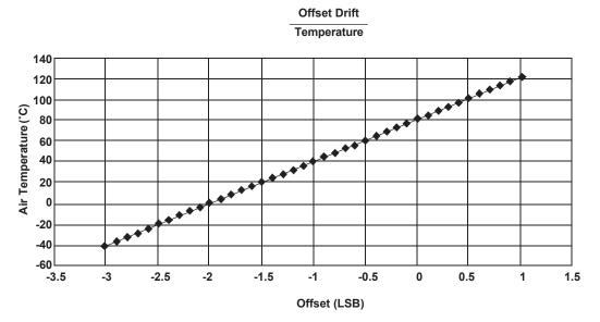
Figure 12. Offset Drift Over Temperature
