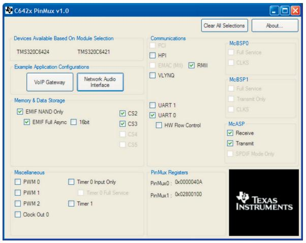
Figure 2. Network Audio Interface Configuration
