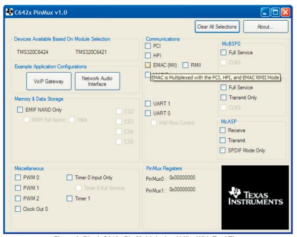
Figure 3. Blank C642x Pin Multiplexing Utility With Tool Tip
