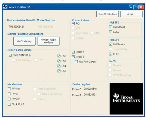
Figure 1. VoIP Gateway Configuration
