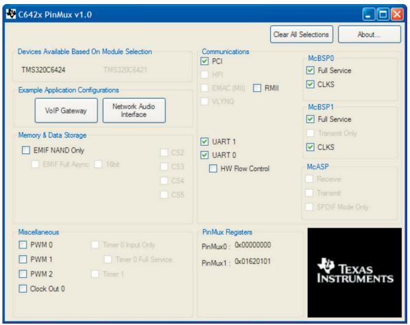
Figure 4. Selecting PCI and Serial Ports
