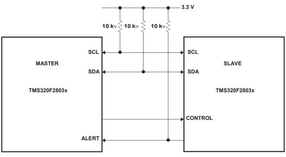
Figure 5. Example Project Setup: F2803x Master and Slave
