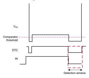
Figure 3-1. Body Diode Conduction Time Detection
