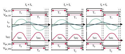
Figure 1-1. Desired SR Driving Signal Under Different f<sub>S</sub>
