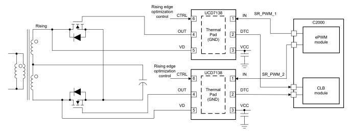
Figure 2-1. C2000 and UCD7138 System Diagram
