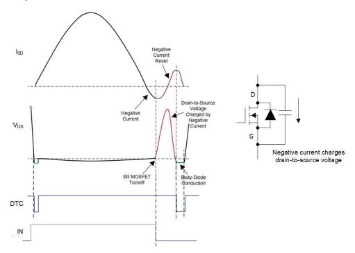
Figure 4-1. SR Drain-to-Source Voltage Shoot Up
