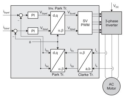
Figure 7. Basic Scheme of FOC for ACI Motor
