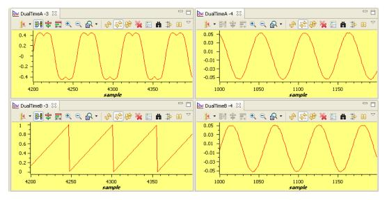
Figure 23. Svgen\_dq1.Ta,Curmod theta, and Phase A and B Current Waveforms
