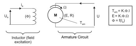
Figure 3. Separated Excitation DC Motor Model
