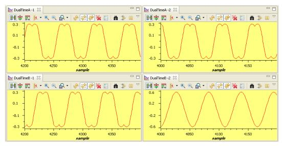
Figure 15. SVGEN Duty Cycle Outputs Ta, Tb, Tc and Tb-Tc
