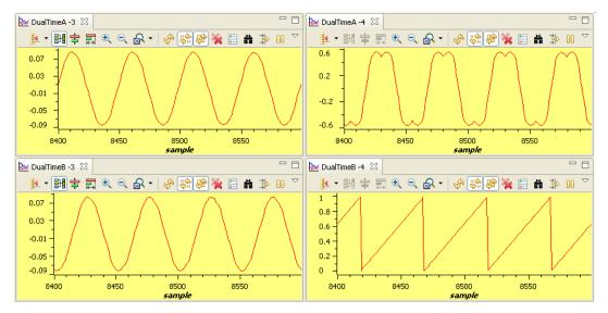
Figure 25. Phase A and B Currents, Svgen\_dq1.Ta, and Curmod θ Waveforms Under 0.5 pu Load, 0.3 pu Speed
