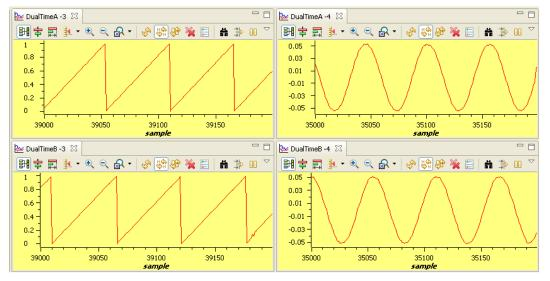
Figure 21. Measured theta, rg1.Out, Phase A and B Current Waveforms
