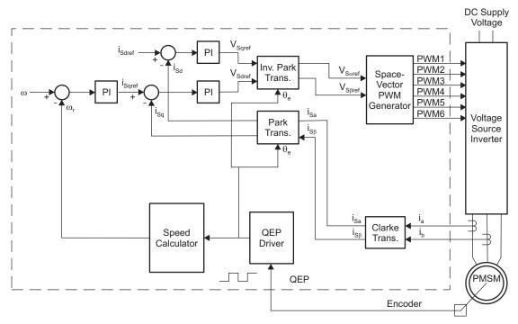
Figure 9. Overall Block Diagram of Sensored Field Oriented Control
