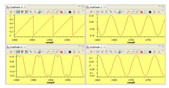
Figure 24. Measured theta, svgen Duty Cycle, and Phase A and B Current Waveforms Under 0.33 pu Load and 0.3 pu Speed
