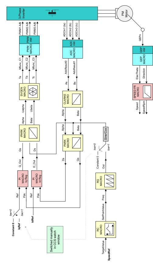
Figure 22. Level 3 - Incremental System Build Block Diagram
