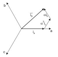
Figure 4. Stator Current Space Vector and Its Component in (a,b,c)
