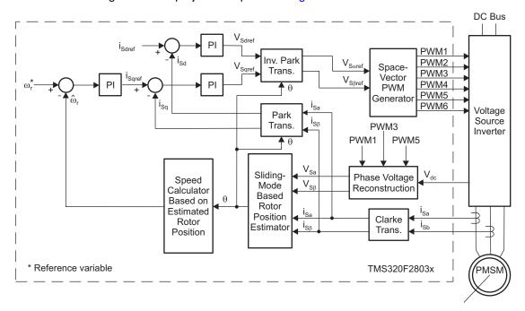
Figure 9. Overall Block Diagram of Sensorless Field Oriented Control of PMSM
