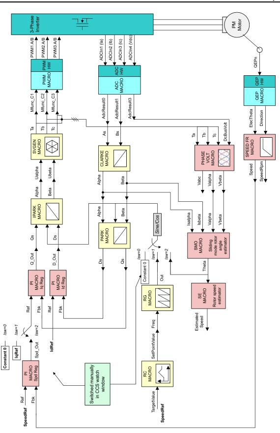
Figure 25. Level 5A - Incremental System Build Block Diagram
