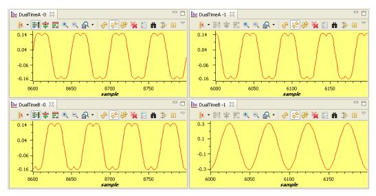
Figure 15. Output of SVGEN, Ta, Tb, Tc and Tb-Tc Waveforms
