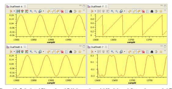
Figure 18. Calculated Phase A and B Voltages by volt1 Module, rg1.Out and svgen\_dq1.Ta
