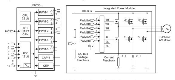
Figure 10. A 3-ph Induction Motor Drive Implementation
