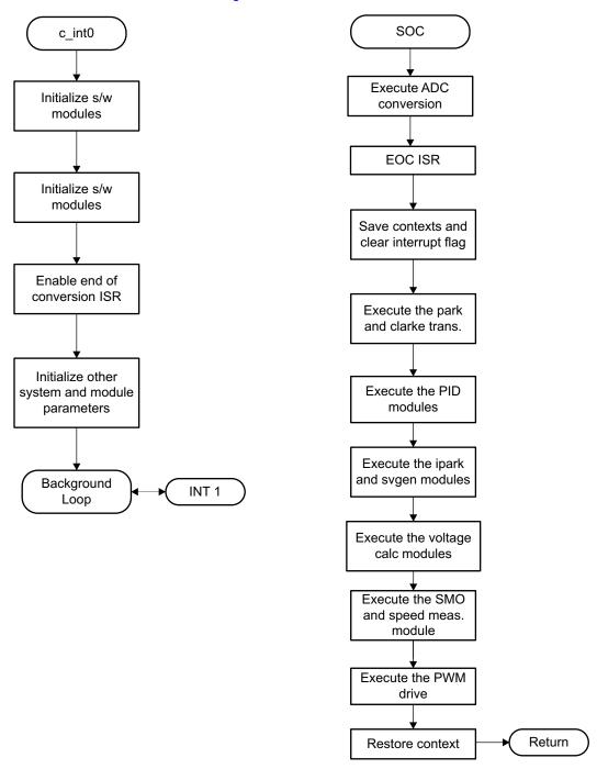
Figure 11. System Software Flowchart
