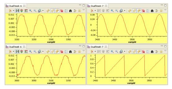
Figure 27. Waveforms of Phase A and B Currents, Calculated Phase A Voltage, and Estimated theta by SMO Under No-Load and 0.3pu Speed
