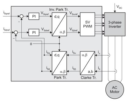
Figure 7. Basic Scheme of FOC for AC Motor
