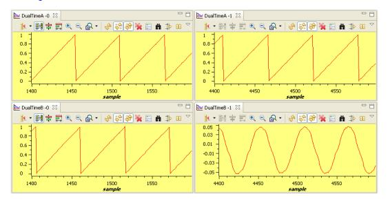
Figure 23. Measured theta, Estimated theta (SMO), rg1.Out and Phase A Current
