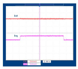
Figure 29. Flux and Torque Components of the Stator Current in the Synchronous Reference Frame Under 0.33 pu Step-Load and 0.5 pu Speed Monitored From PWMDAC Output
