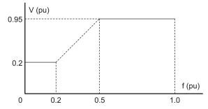
Figure 12. V/Hz Profile Configuration Used in This System
