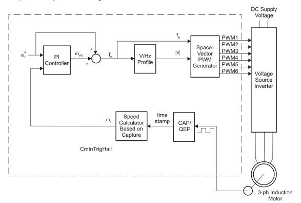
Figure 7. A 3-ph Induction Motor V/Hz Drive Implementation
