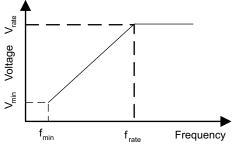
Figure 6. Modified V/Hz Profile
