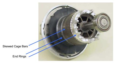
Figure 1. Induction Motor Rotor
