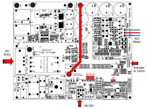
Figure 9. Using AC Power to Generate DC Bus Power
