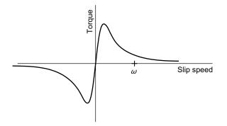
Figure 5. Torque Versus Slip Speed of an Induction Motor With Constant Stator Flux
