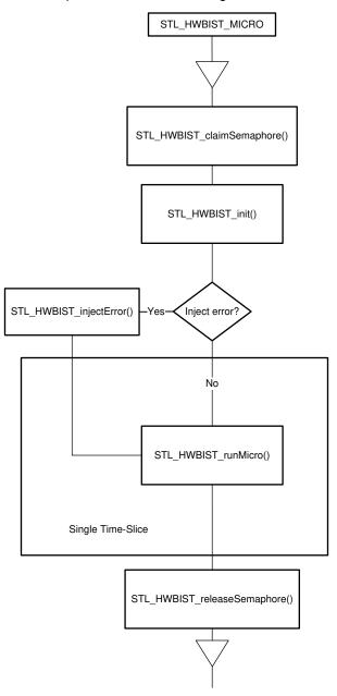
Figure 2-2. Flow Chart of Time-Sliced Micro-Run Execution
