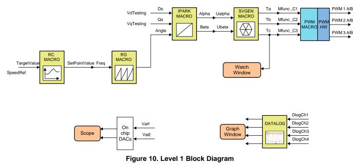
The block diagram of the system built in BUILD LEVEL 1 is shown in Figure 10. At this step, keep the motor disconnected. This section describes the steps for a "minimum" system check-out, which confirms operation of system interrupt, the peripheral and target independent I\_PARK\_MACRO (inverse park transformation) and SVGEN MACRO (space vector generator) modules and the peripheral dependent PWM MACRO (PWM initializations and update) modules.
