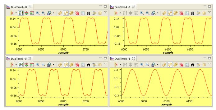
Figure 12. Output of SVGEN, Ta, Tb, Tc and Tb-Tc Waveforms
