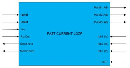
Figure 2. Fast Current Loop (FCL) Library Block Diagram
