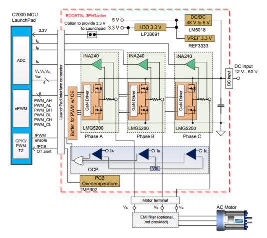
Figure 7. BOOSTXL-3PhGaNInv Functional Block Diagram
