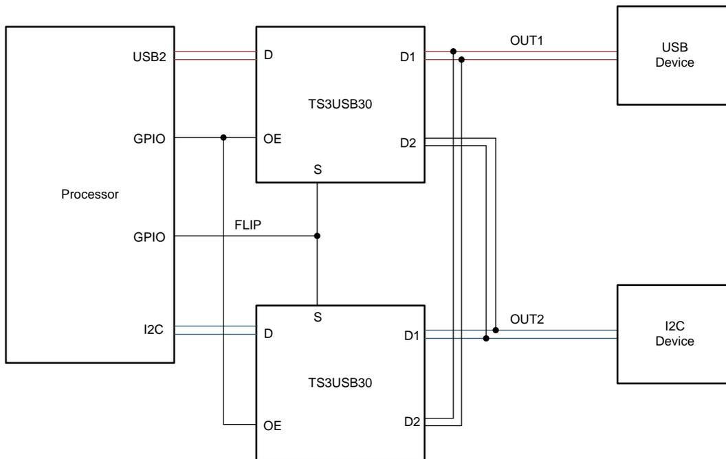
Figure 3. 2:2 Differential Fan Out Switch Schematic
