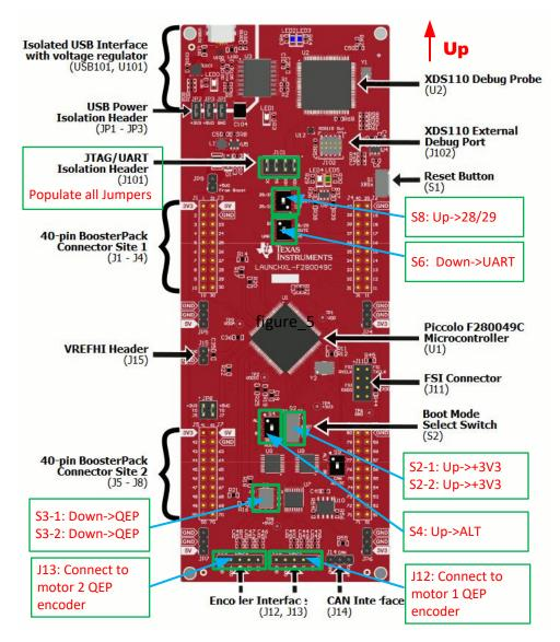
Figure 5. Layout of LAUNCHXL-F280049C and Switches Setting
