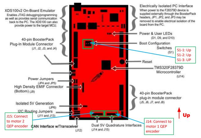
Figure 4. Layout of LAUNCHXL-F28379D and Switches Setting
