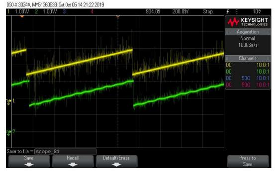
Figure 31. DACs in Scope Plot of Reference Position to Servo and Feedback Position
