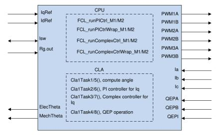
Figure 3. Fast Current Loop Block Diagram
