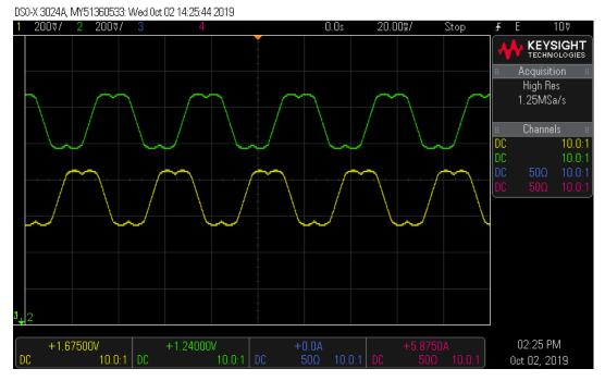
Figure 21. DAC Outputs Showing Ta, Tb Waveform
