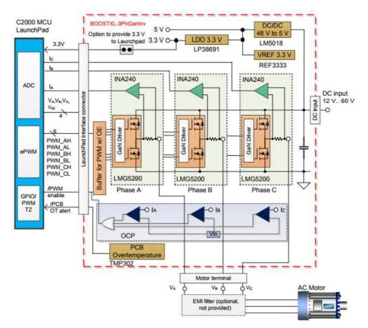
Figure 6. BOOSTXL-3PhGaNInv Functional Block Diagram
