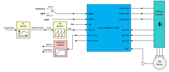
Figure 25. Level 3 Block Diagram Showing Inner Control Loop - FCL
