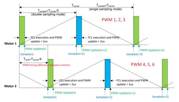
Figure 2. Motor Phase Current Sampling and PWM Update for Dual Motor
