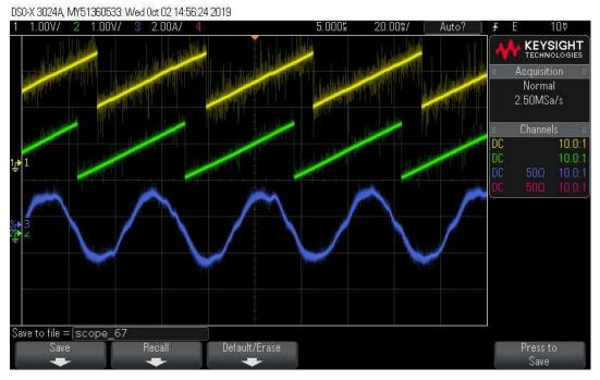
Figure 23. DAC Outputs on Scope Showing Reference Angle and Rotor Position
