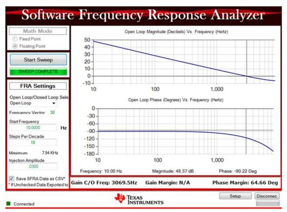
Figure 38. SFRA Open Loop Bode Plots of the Current Loop - Current Feedback With High SNR
