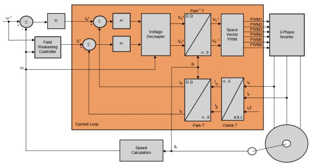
Figure 1. Basic Scheme of FOC for AC Motor
