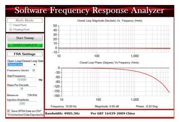
Figure 36. SFRA Open Loop Bode Plots of the Current Loop Showing Magnitude and Phase Angle
