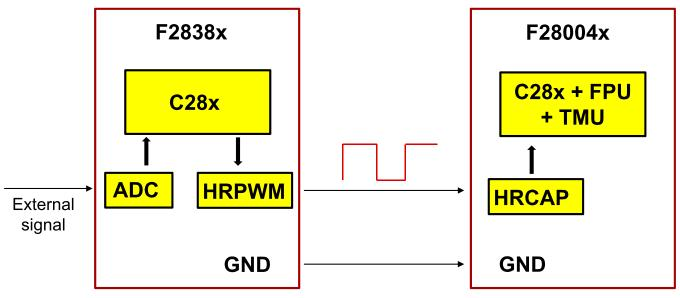
Figure 2. Cross Device Data Transfer
