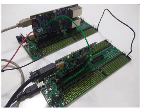
Figure 4. Test Setup for Cross Device Data Transfer
