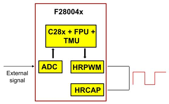
Figure 3. Device Loopback Data Transfer
