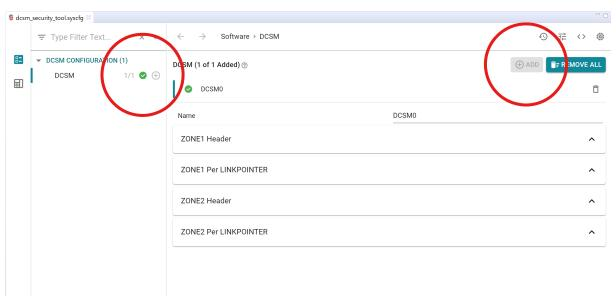
Figure 4-1. Adding a SECURITY Module to Project
