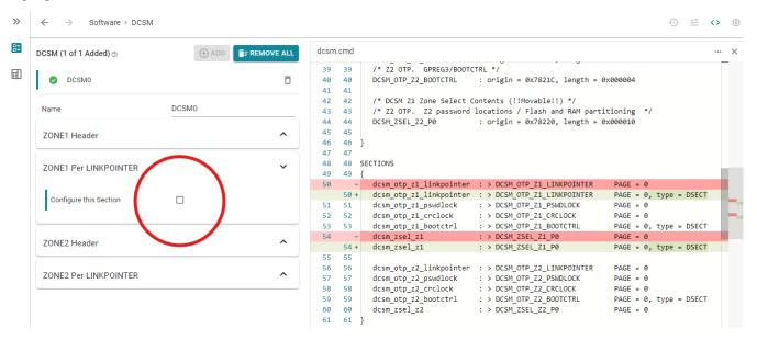
Figure 5-3. dcsm.cmd Highlighting the Changes
