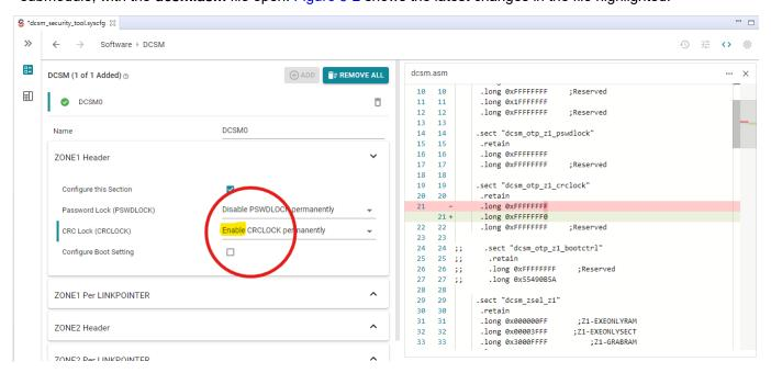
Figure 5-2. dcsm.asm Highlighting the Changes
