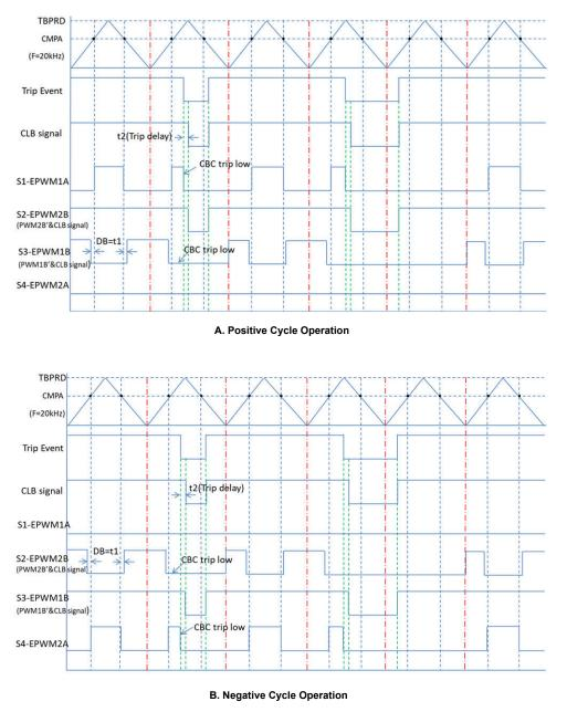
Figure 2-1. Expected EPWM Protection Logic With CLB
