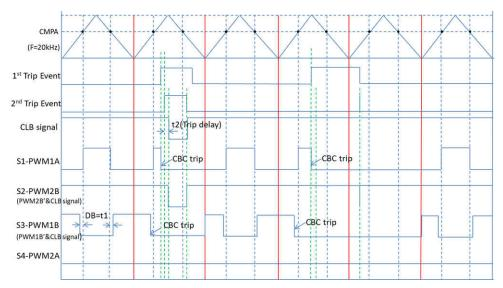
Figure 5-3. Updated EPWM Protection Logic With CLB for 2 Level Protection Scheme
