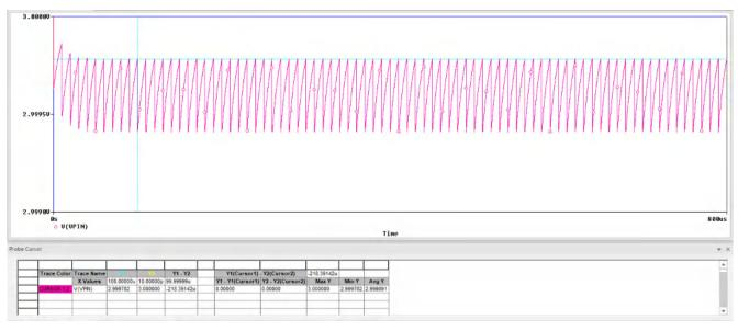
Figure 2-5. Simulation Results for  $100\Omega$   $R_s$  and 100 kHz Sample Rate
