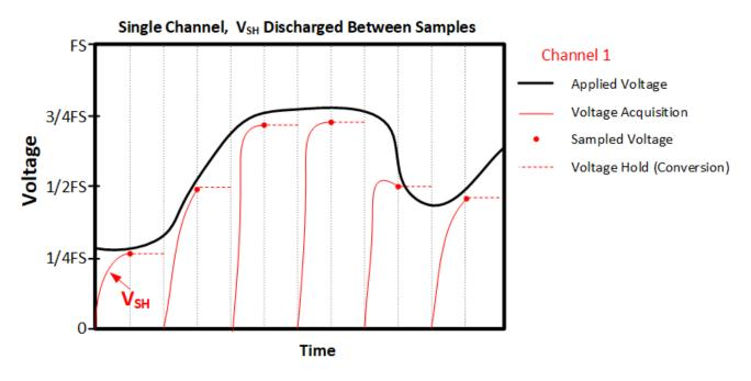
Figure A-3. Sequence of Samples With C<sub>H</sub> Discharged Between Conversions
