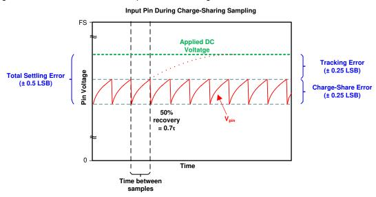
Figure 2-7. Charge Sharing Steady State With DC Input
