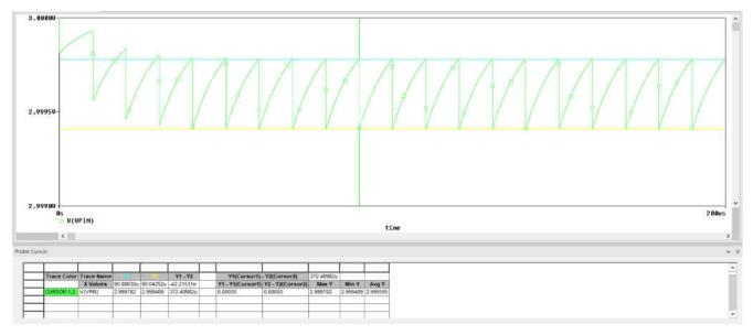
Figure 4-14. Settling Error Component Measurement
