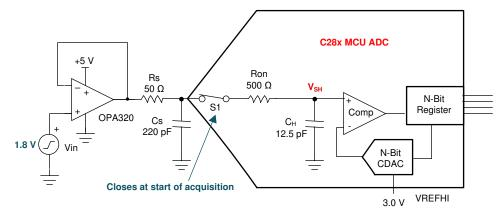
Figure 2-1. High Speed ADC Driving Circuit
