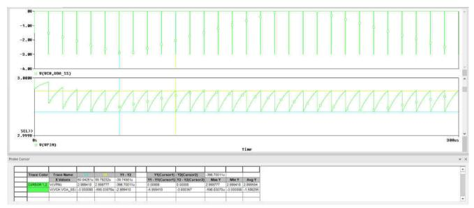
Figure 4-13. Settling Error Measurement
