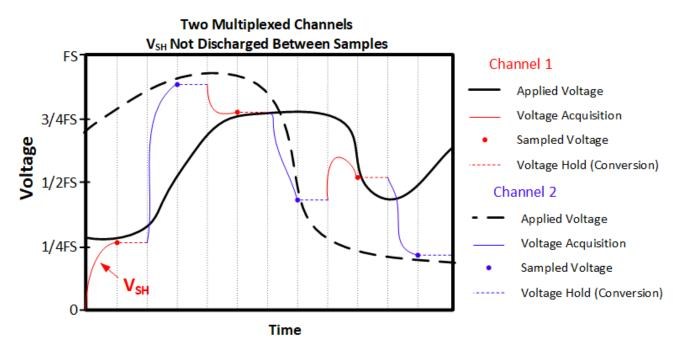
Figure A-4. Sequence of Multiplexed Samples
