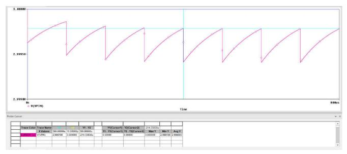
Figure 2-6. Simulation Results for  $1k\Omega R_s$  and 10kHz Sample Rate
