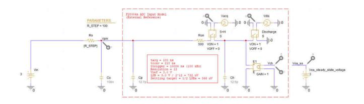
Figure 4-1. Simulation Schematic (No Op-Amp)
