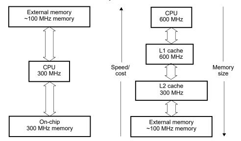
Figure 1–1. Flat Versus Hierarchical Memory Architecture
