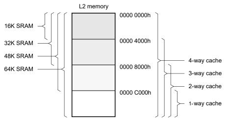
Note that when the L2 cache size is increased the memory is taken from the high memory addresses. Other configurations are set by adjusting the cache size in Figure 2–1 and Figure 2–2. Therefore, the corresponding CACHE setL2Mode() calls and MEMORY definitions are following.
