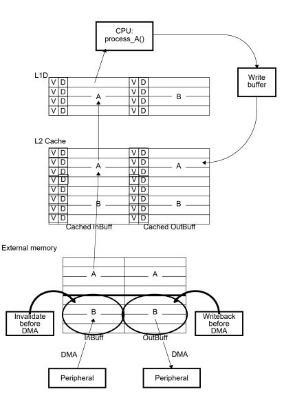
To maintain coherence, you have to imitate for external memory what the cache controller does for L2 SRAM accesses. Whenever data is written to an input buffer, the cache controller would *invalidate* the corresponding line in the cache. Similarly, here all the lines in L1D *and* L2 cache that map to the external memory input buffer have to be invalidated before the DMA transfer starts. This way the CPU will reallocate these lines from external memory next time the input buffer is read.
