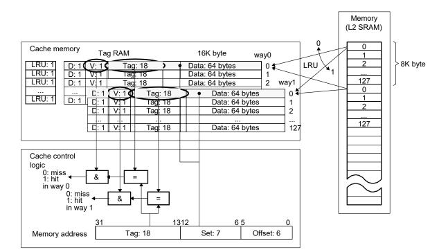
Figure 1–7. C64x L1D Architecture
