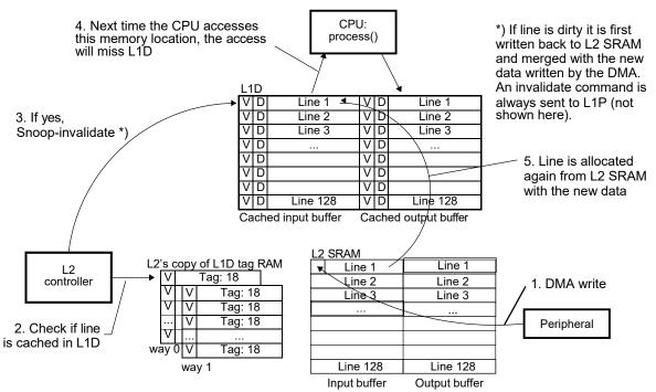
The procedure for a DMA read is shown in Figure 2–9 and is:
