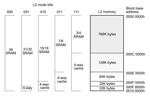
Note that when the L2 cache size is increased the memory is taken from the high memory addresses. Other configurations are set by adjusting the cache size in Figure 2–4 and Figure 2–5. Therefore, the corresponding CACHE setL2Mode() calls and MEMORY definitions are following.
