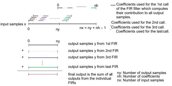
While new input samples replace old ones in cache, this does not matter as long as the coefficients are retained. If the coefficients are kept in one way and the input samples in the other (the size of the coefficient subset is not larger than one way of L1D), the coefficients will not be evicted by input samples. The behavior of the LRU replacement scheme automatically ensures that the lines which are not reused are replaced, leaving the ones that are reused in the cache.
