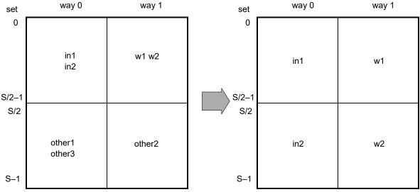
Figure 3–9. Mapping of Arrays to L1D Sets for Dot Product Example
