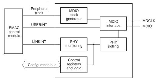
Figure 9. MDIO Module Block Diagram
