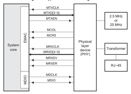
Figure 2. Typical Ethernet Configuration
