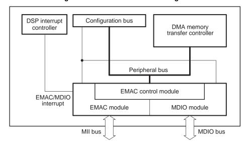
Figure 1. EMAC and MDIO Block Diagram
