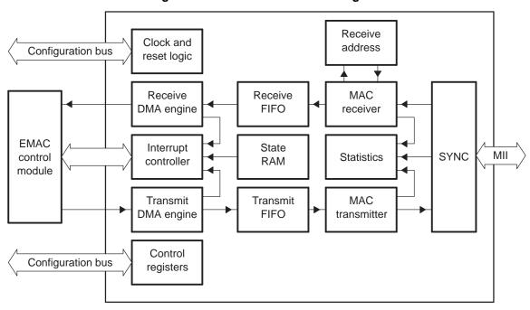
Figure 10. EMAC Module Block Diagram
