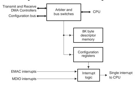
Figure 8. EMAC Control Module Block Diagram
