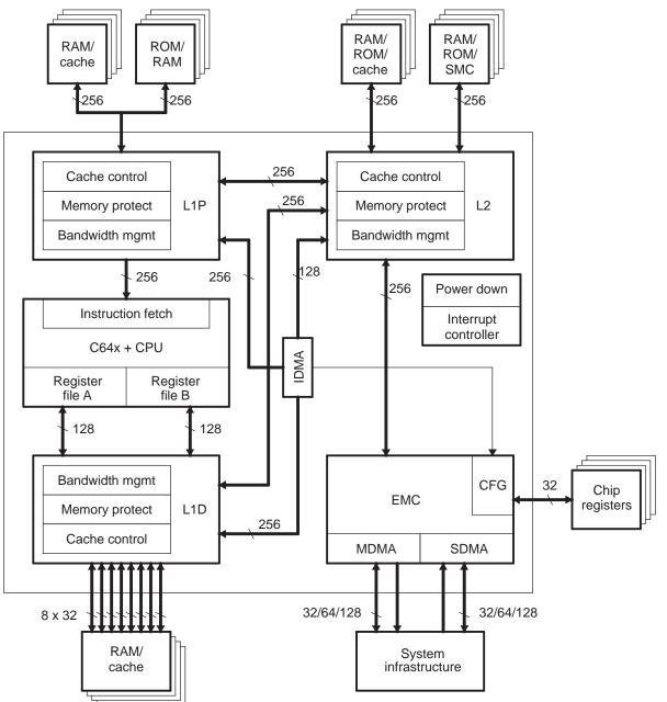
Figure 1. DSP Subsystem Block Diagram
