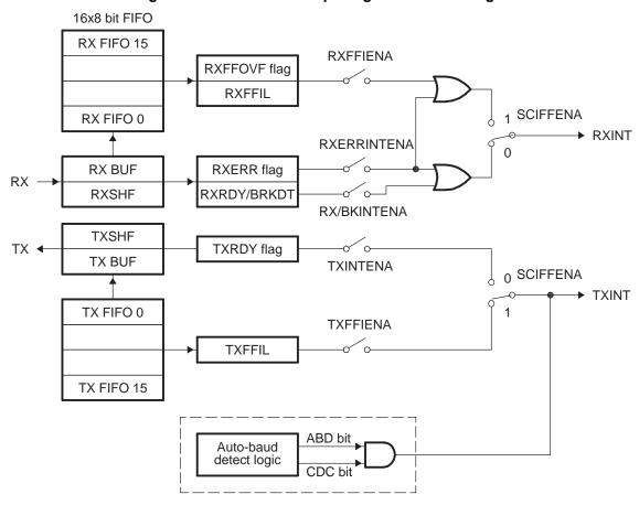
Figure 10. SCI FIFO Interrupt Flags and Enable Logic
