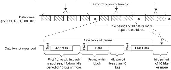
Figure 4. Idle-Line Multiprocessor Communication Format
