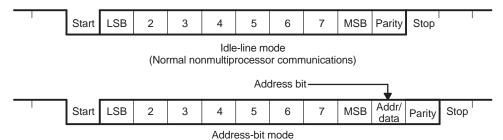
To program the data format, use the SCICCR register. The bits used to program the data format are shown in Table 4.
