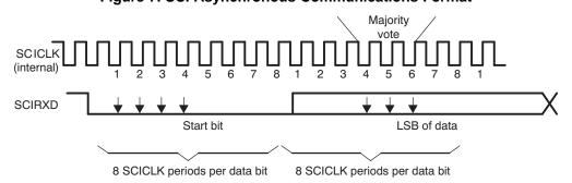
Figure 7. SCI Asynchronous Communications Format
