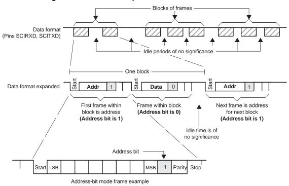
Figure 6. Address-Bit Multiprocessor Communication Format
