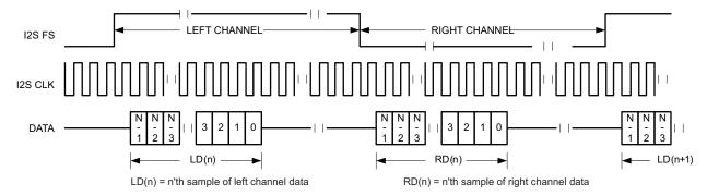
Figure 8. Timing Diagram for I2S Mode
