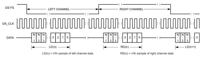
Figure 9. Timing Diagram for I2S Mode with Inverse Bit-Clock Polarity
