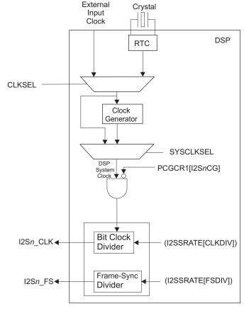
Figure 2. Inter-IC Sound Clock Control Diagram
