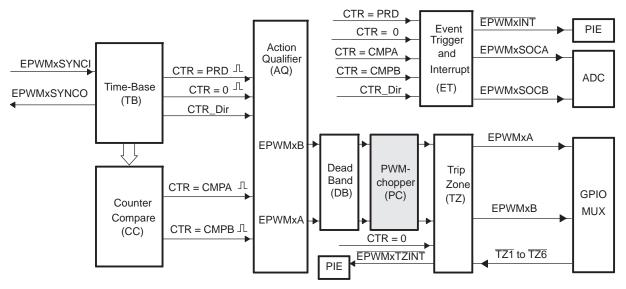
The PWM-chopper submodule allows a high-frequency carrier signal to modulate the PWM waveform generated by the action-qualifier and dead-band submodules. This capability is important if you need pulse transformer-based gate drivers to control the power switching elements.
