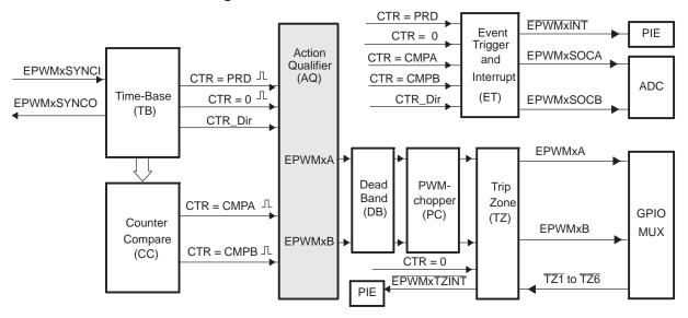
The action-qualifier submodule has the most important role in waveform construction and PWM generation. It decides which events are converted into various action types, thereby producing the required switched waveforms at the EPWMxA and EPWMxB outputs.
