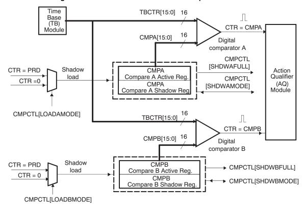
The key signals associated with the counter-compare submodule are described in Table 6.
