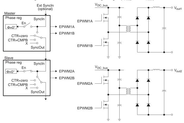
Figure 53. Control of Two Half-H Bridge Stages (F<sub>PWM2</sub> = N x F<sub>PWM1</sub>)
