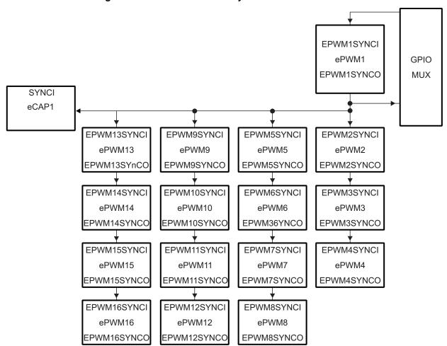
Figure 8. Time-Base Counter Synchronization Scheme 2
