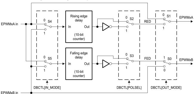
Figure 31. Configuration Options for the Dead-Band Submodule
