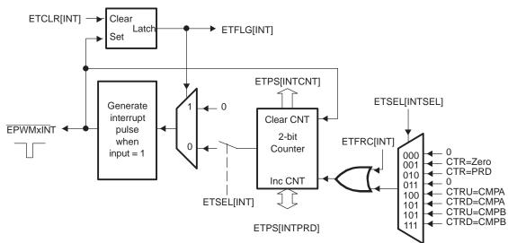
Figure 44. Event-Trigger Interrupt Generator
