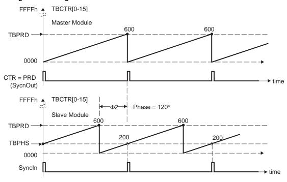
Figure 58. Timing Waveforms Associated With Phase Control Between 2 Modules
