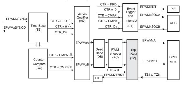
Each ePWM module is connected to six  $\overline{TZn}$  signals ( $\overline{TZ1}$  to  $\overline{TZ6}$ ) that are sourced from the GPIO MUX. These signals indicate external fault or trip conditions, and the ePWM outputs can be programmed to respond accordingly when faults occur.
