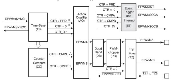
Figure 41. Event-Trigger Submodule
