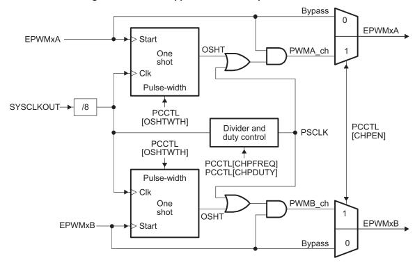
Figure 34. PWM-Chopper Submodule Operational Details
