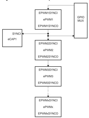
Figure 7. Time-Base Counter Synchronization Scheme 1
