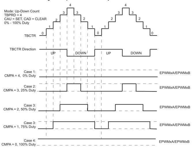
Figure 23. Up-Down-Count Mode Symmetrical Waveform
