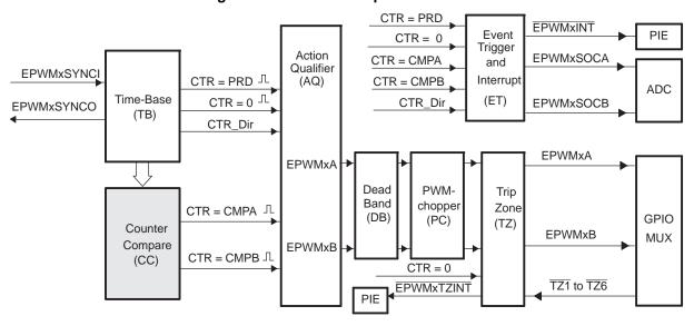
Figure 15 shows the basic structure of the counter-compare submodule.
