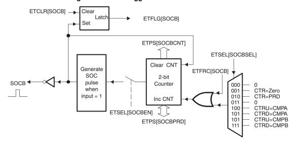
Figure 46. Event-Trigger SOCB Pulse Generator
