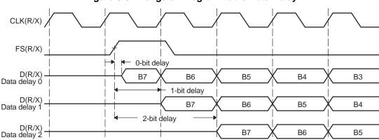
Figure 8-6. Range of Programmable Data Delay
