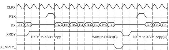
Figure 4-8. Underflow Prevented in the McBSP Transmitter
