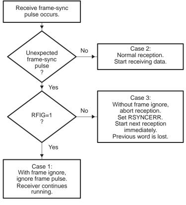
Figure 4-3. Possible Responses to Receive Frame-Synchronization Pulses
