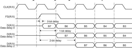
Figure 7-4. Range of Programmable Data Delay
