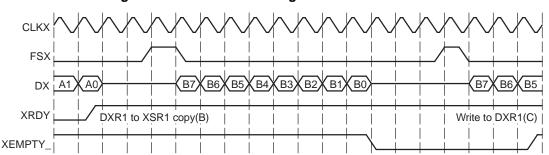
Figure 4-7. Underflow During McBSP Transmission
