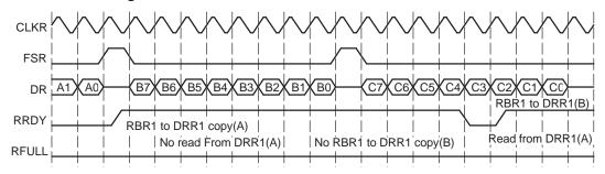
Figure 4-2. Overrun Prevented in the McBSP Receiver
