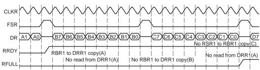
Figure 4-1. Overrun in the McBSP Receiver
