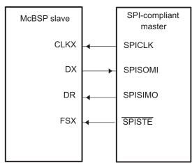
Figure 6-7. SPI Interface With McBSP Used as Slave
