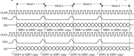
Figure 10-3. 8-Bit Data Words Transferred at Maximum Packet Frequency
