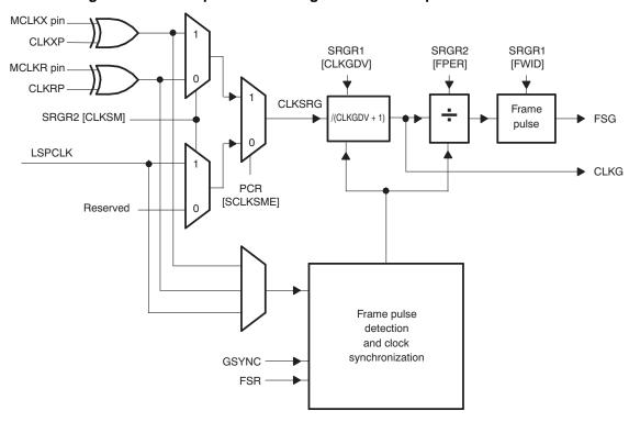
The source clock for the sample rate generator (labeled CLKSRG in the diagram) can be supplied by the LSPCLK, or by an external pin (MCLKX or MCLKR). The source is selected with the SCLKME bit of PCR and the CLKSM bit of SRGR2. If a pin is used, the polarity of the incoming signal can be inverted with the appropriate polarity bit (CLKXP of PCR or CLKRP of PCR).
