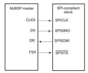
Figure 6-6. SPI Interface with McBSP Used as Master
