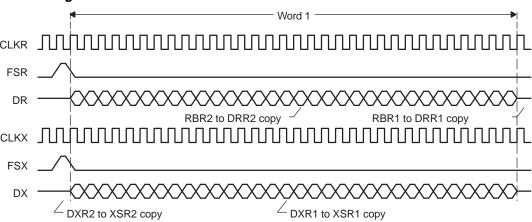
Figure 10-2. One 32-Bit Data Word Transferred To/From the McBSP
