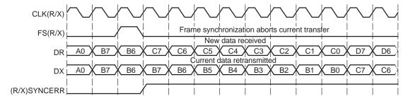
In contrast with Figure 8-1, Figure 8-2 shows McBSP operation when unexpected frame-synchronization signals are ignored (when (R/X)FIG = 1). Here, the transfer of word B is not affected by an unexpected frame-synchronization pulse.
