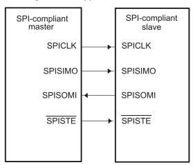
Figure 6-1. Typical SPI Interface
