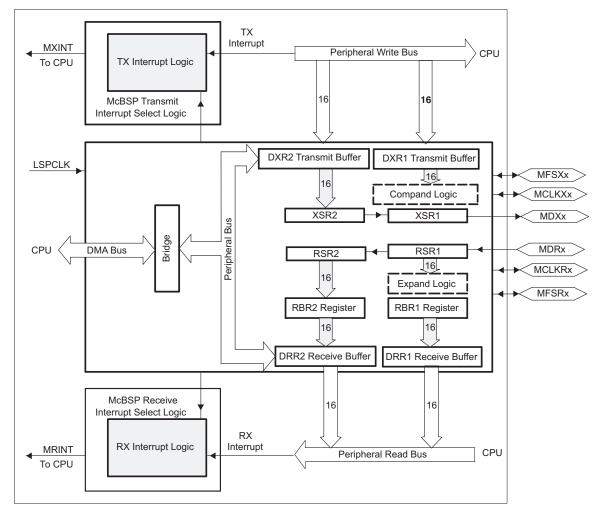
Figure 1-1. Conceptual Block Diagram of the McBSP
