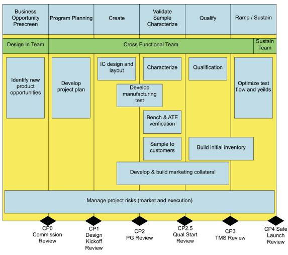
Figure 2. TI Standard MCU Automotive QM Development Process
