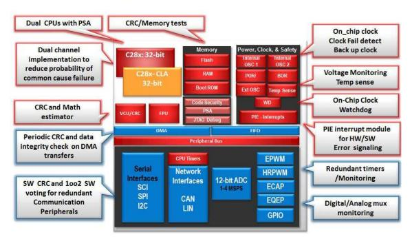
Figure 3. C2000 MCU Piccolo F2806x With Safety Features in Software
