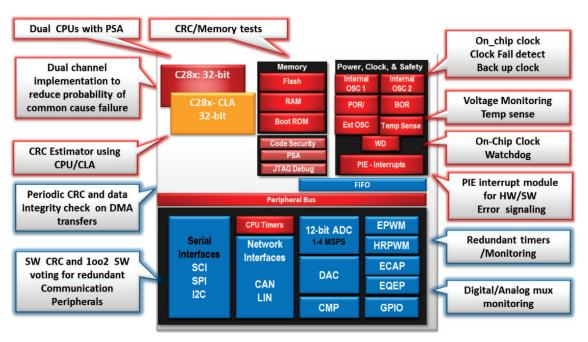
C28x CPU + CLA with Control & Analog Subsystem
