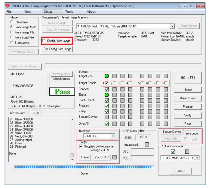
NOTE: This figure shows the From Image Mem. mode (top left corner). The Config. from Image option is disabled in this example, allowing the user to change various but not all configuration settings from the image. The configuration options that can be changed are highlighted in red. One of the options that cannot be changed, for example, is the target processor type.
