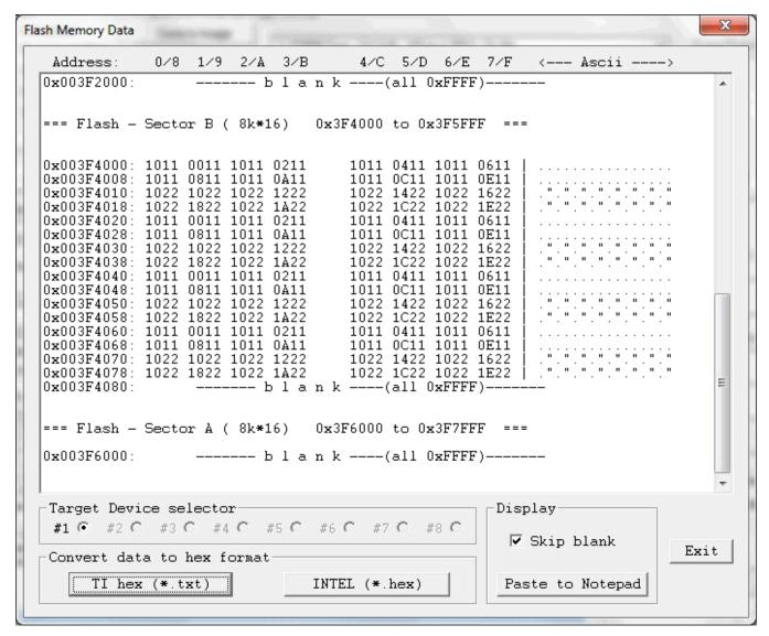
NOTE: This window displays the code addresses on the left side, data in hex format in the center column, and the same data in ASCII format in the right column.
