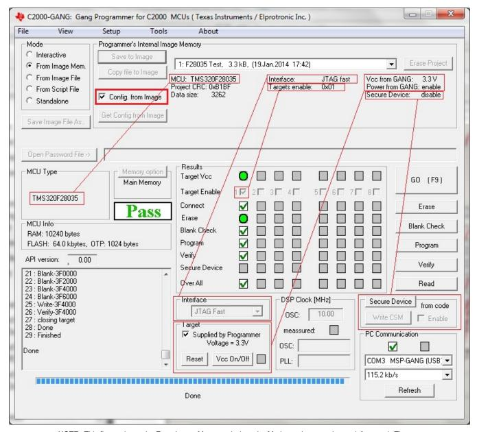
NOTE: This figure shows the From Image Mem. mode (see the Mode section near the top left corner). The user can load an image from C2000 Gang Programmer internal memory. Saved images contain all configuration necessary for programming and all code files. An image can be created using the Interactive Mode and saved to the programmer. One of 16 different images can be selected from internal memory, or one image from each external SD-Card can be used.
