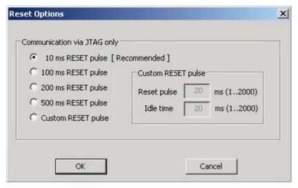
NOTE: This window lets the user specify the duration of the reset pulse coming from the C2000 Gang Programmer to the target device. Depending on the hardware implementation, a longer reset pulse might be required.
