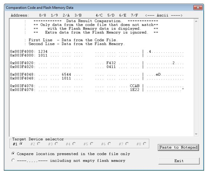
NOTE: Only words that differ are shown. The selected option on the bottom of the figure specifies that only memory segments corresponding to the code file should be compared. The second option, if selected, performs the comparison and shows any remaining contents of flash memory that do not correspond to the code file.
