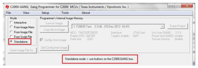
NOTE: This figure uses the Standalone mode (see the Mode section near the top-left corner). All GUI options are disabled; the C2000 Gang Programmer can only be operated using physical controls on the programmer itself. Standalone mode allows the user to program a target device using an image either from internal memory (up to 16 different images), or an external SD-Card, without the use of a desktop or laptop computer.
