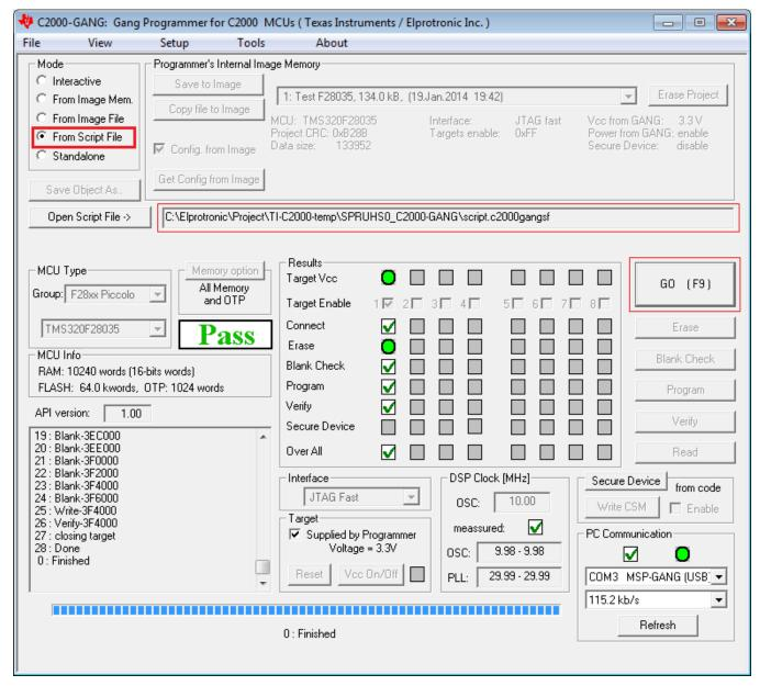
NOTE: This figure shows the From Script mode (see the Mode section near the top left corner). A script file is selected using the Open Script File button and it specifies all configuration options, and the code files to be used for programming. In addition, the script can call individual functions, such as Program or Verify, in the order specified by the programmer.
