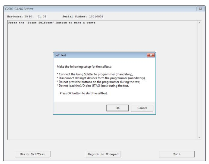
NOTE: Use the C2000 Gang Programmer selftest capability to check the integrity of the hardware. Before beginning the test, make sure that no target MCUs are connected to the C2000 Gang Programmer.
