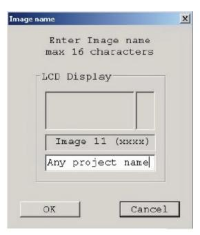
NOTE: The image name is limited to 16 characters. This name is shown on the LCD display of the C2000 Gang Programmer and Image pulldown menu in the GUI.
