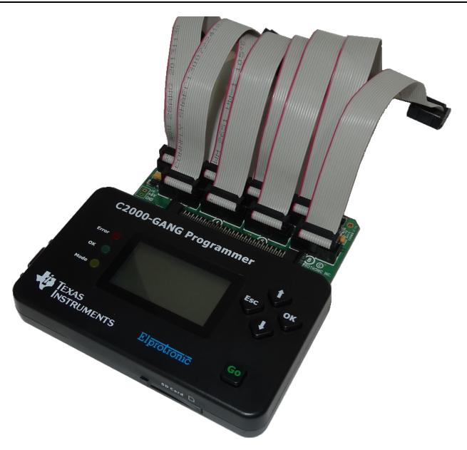
Figure 1-1. Top View of the C2000 Gang Programmer
