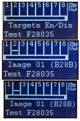
Figure 2-10. Target Enable or Disable Option
