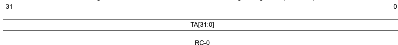
Figure 14-13. Transmission-Acknowledge Register (CANTA)
