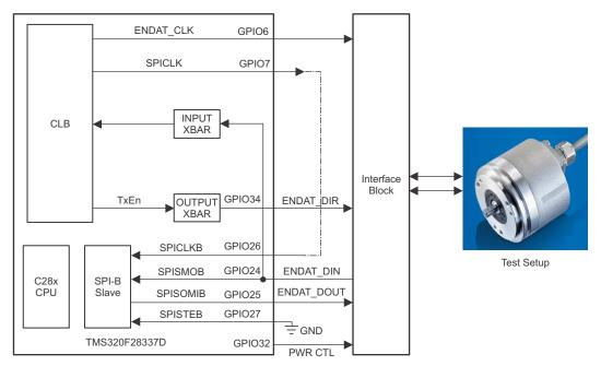
Figure 2. EnDat Implementation Diagram Inside TMS320F28379D
