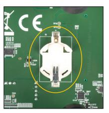
Note: This EVM is designed for optional use with a removable CR2032 UL recognized lithium battery (not supplied). Always use the CR2032VP Energizer 3V Lithium coin cell battery or similar CR2032 UL recognized battery with Nominal Voltage 3.0 Volts, Capacity 235mAh
