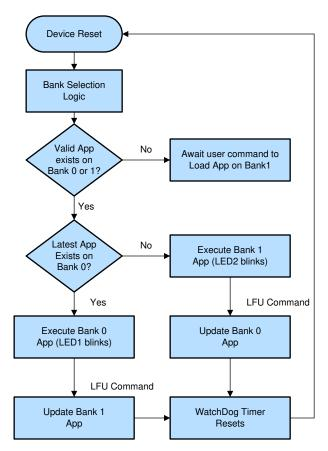
Figure 6-15. LFU Code Flow Diagram
