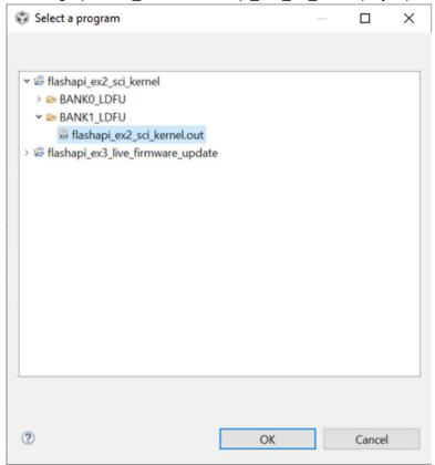
Figure 6-8. Selecting Kernel to Load to Flash Bank 1
