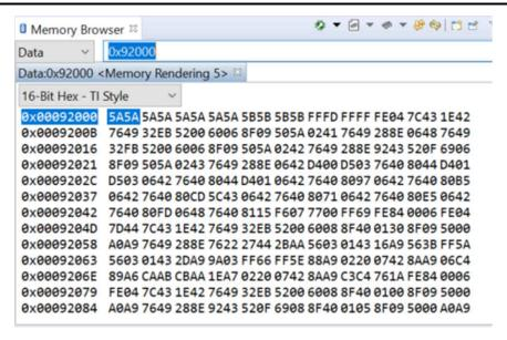
Figure 6-7. CCS Memory Browser View to Verify Successful Programming of Application on Bank 1
