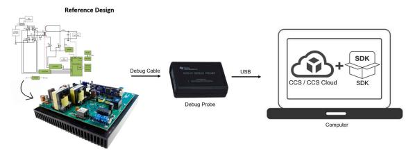
Figure 2-4. C2000 Advanced Level Ecosystem Diagram
