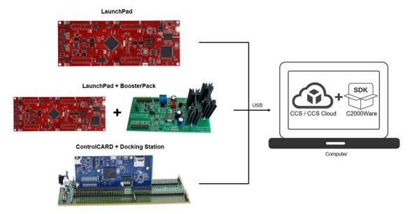
Figure 2-2. C2000 Entry Level Ecosystem Diagram
