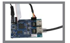
Connect the recommended power supply (CUI Inc. SMI18-5-V-P5, procurable at: http://www.digikey.com/product-detail/en/ cui-inc/SMI18-5-V-P5/102-3571-ND/5415042) or equivalent (Output voltage/current: 5 Volts DC ± 10% @ 1.2 Amps; Output connector: 2.1-mm ID, 5.5-mm OD barrel plug, center positive) power supply to J8 on the ICE board. Apply power to the power supply to power up the ICE board. Do not hot plug the 5-V supply into the ICE board.
