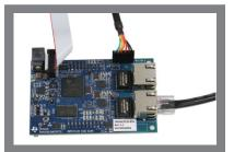
Connect a CAT5 Ethernet cable from a PC running TwinCAT software to ECAT IN/ PHY1 (J6) of the ICE board. If you have multiple ICE boards in a chain, please connect another CAT5 Ethernet cable from ECAT OUT/PHY2 (J7) to PHY1 of the next ICE board. PHY2 of the last ICE board in the chain is left open.
