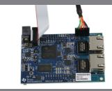
Connect the pin header connector of included TTL-232R-3V3 serial cable to J3 on the ICE board. Ensure that pin 1 of the serial cable (black wire, marked with a triangle) is connected to pin 1 of J3, which is indicated by a dot on the silk screen. Datasheet for this cable can be found at:
