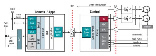
Figure 4: Multi-axis drive with real-time Ethernet
