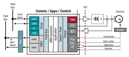
Figure 3: Servo drive with real-time Ethernet
