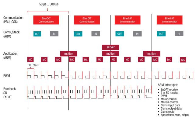
Figure 10: Connected industrial drive control cycle
