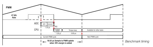
Figure 11: Single-chip drive motor control configuration and benchmark timing on AM437x processors
