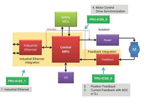
Figure 6: Integrated connected industrial drive building blocks
