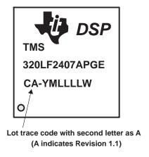
Figure 1. Example, Lot Trace Code for TMS320LF2407A (PGE)
