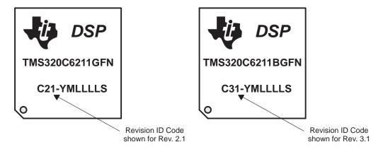
NOTE: Qualified devices are marked with the letters "TMS" at the beginning of the device name, while nonqualified devices are marked with the letters "TMX" or "TMP" at the beginning of the device name.
