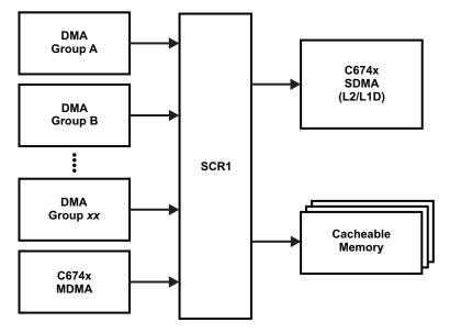
Figure 6. SCR1 System Interconnect
