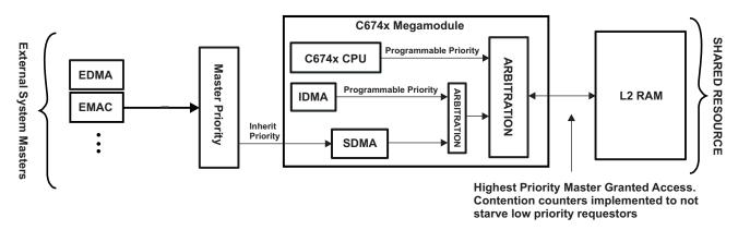
7. Figure 2 shows a high level diagram of the arbitration scheme used for L2 RAM
