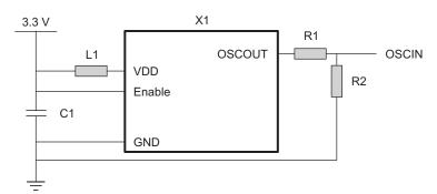
Legend: L1 = ferrite bead; C1 = 0.1 uF; R1 = 165 ohm / 5%; R2 = 100 ohm / 5%
