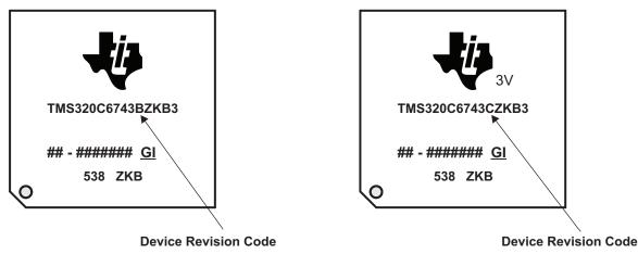
Example, Device Revision Codes for TMS320C6743 (ZKB Package)
