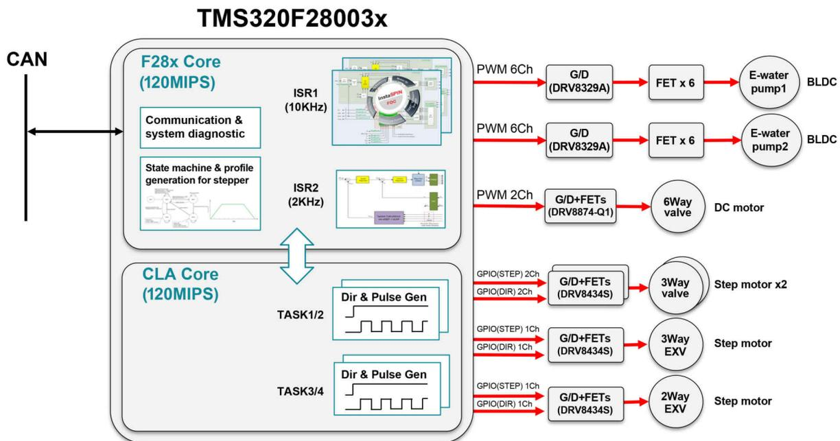
**Figure 2. A Heat-pump System Controlled by a C2000 Real-time MCU**
