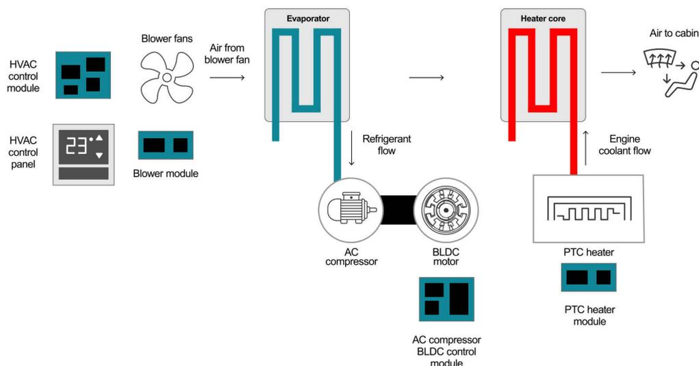
**Figure 1. The Heating and Cooling System in an HEV and EV**
