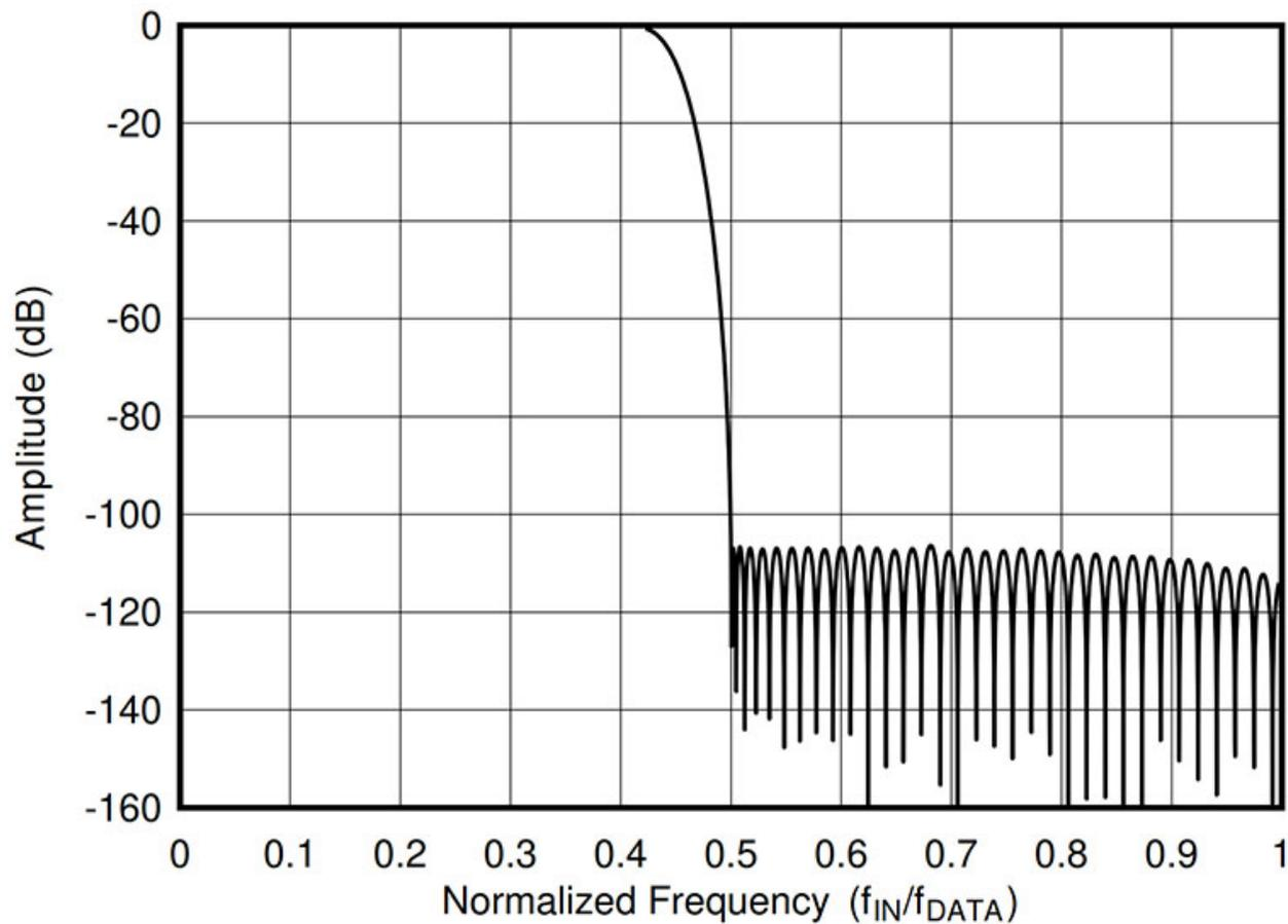
**Figure 3. Wideband ADC Filter Response**
