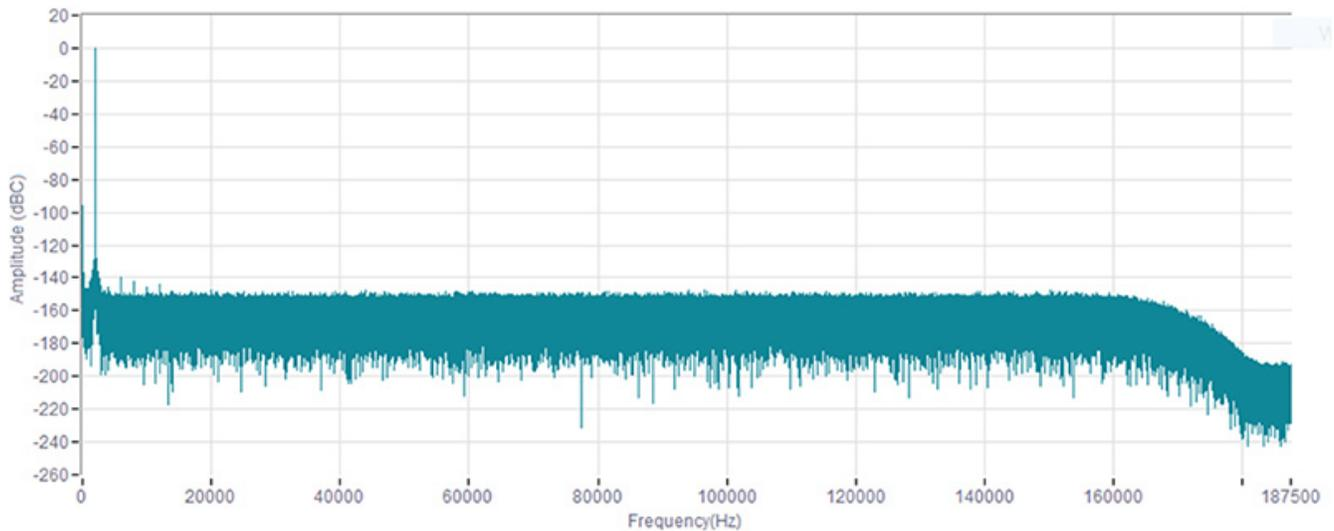
**Figure 2. ADC Spectral Performance**
