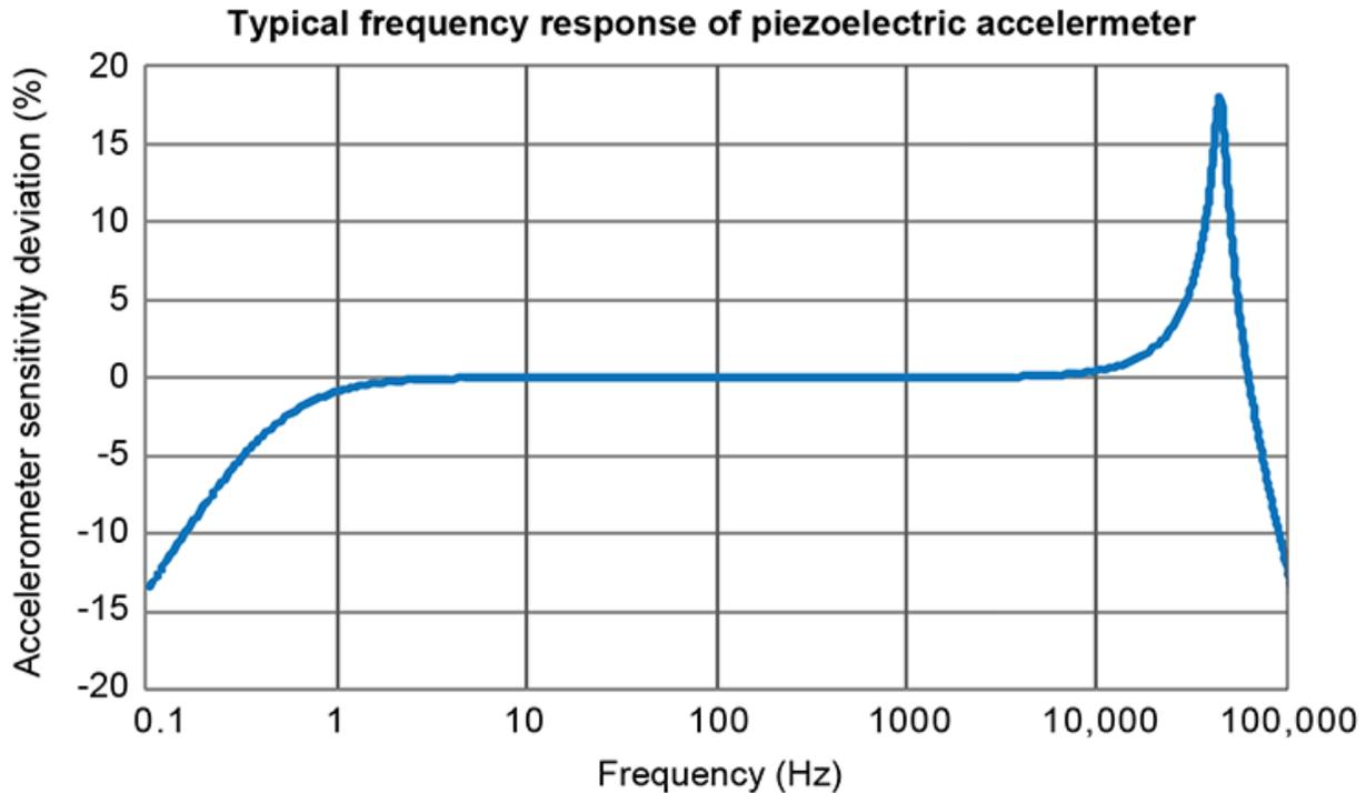
**Figure 4. Typical Piezo Accelerometer with Response Peaking at Resonance**
