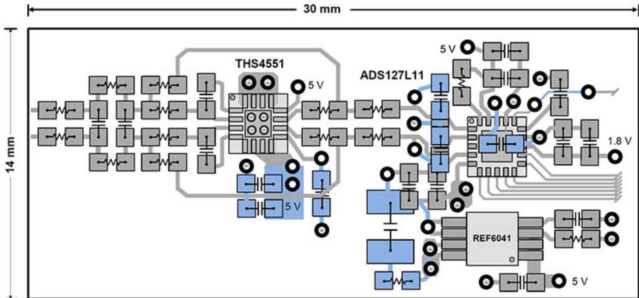
Figure 1. Typical Analog-front-end Printed Circuit Board (PCB) Layout
