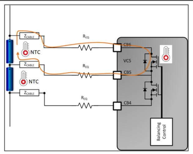
Figure 2. BQ79616-Q1 temperature monitoring locations on the PCB
