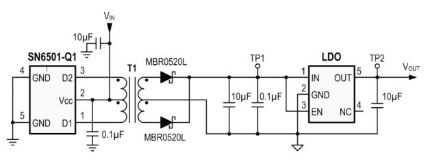
Figure 3. Simple circuit for an isolated power supply with a regulated output
