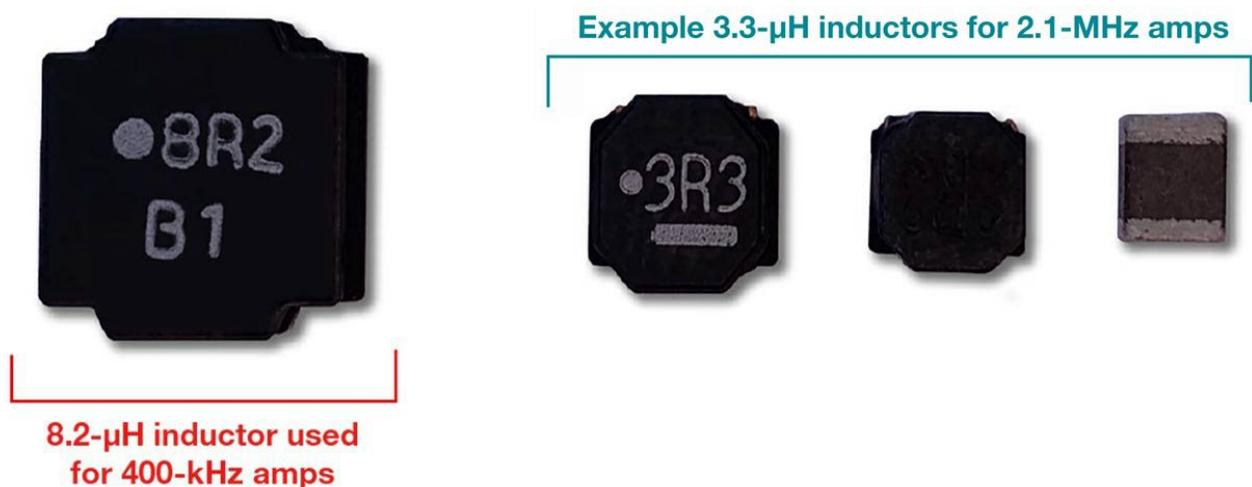
Figure 1. Comparison of Inductor Size vs. Switching Frequency
