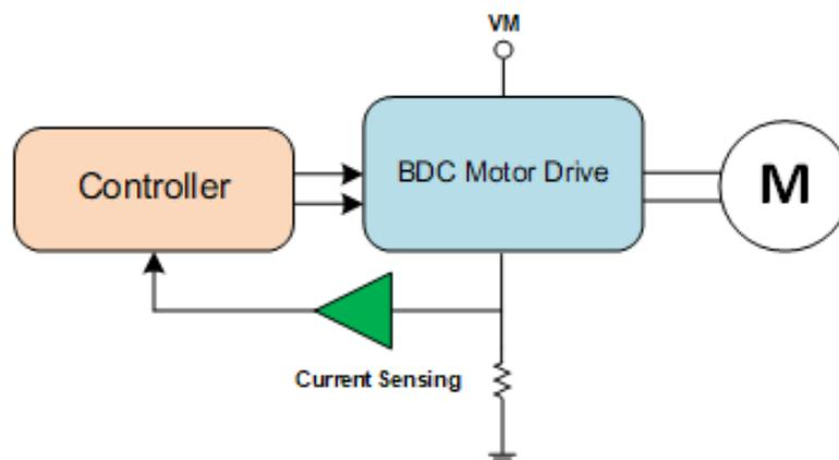
Figure 1. Current-sensing Circuit in a Motor Control System
