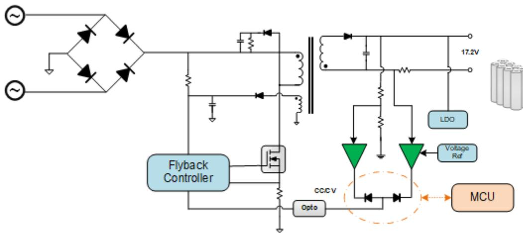
**Figure 2. A Discrete Battery Charger Circuit**
