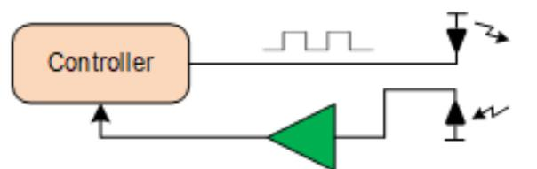
**Figure 6. A Signal Conditioning Circuit for an Infrared LED Receiver**
