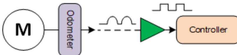
**Figure 4. Buffer for a Robust Logic Output Circuit**
