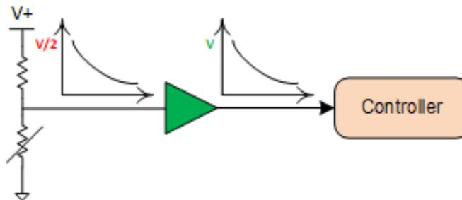
**Figure 3. NTC Thermistor Sensing Circuit**
