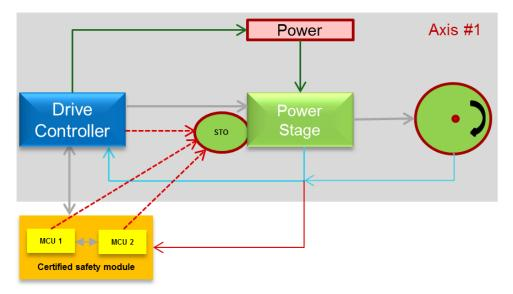
Figure 1. Two-channel functional safety module example
