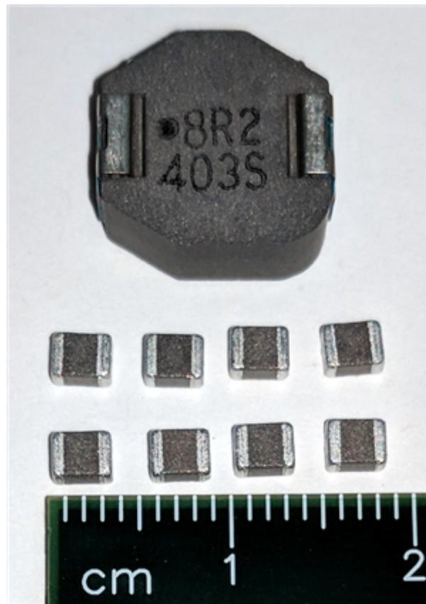
Figure 3. Inductor Size Comparison
