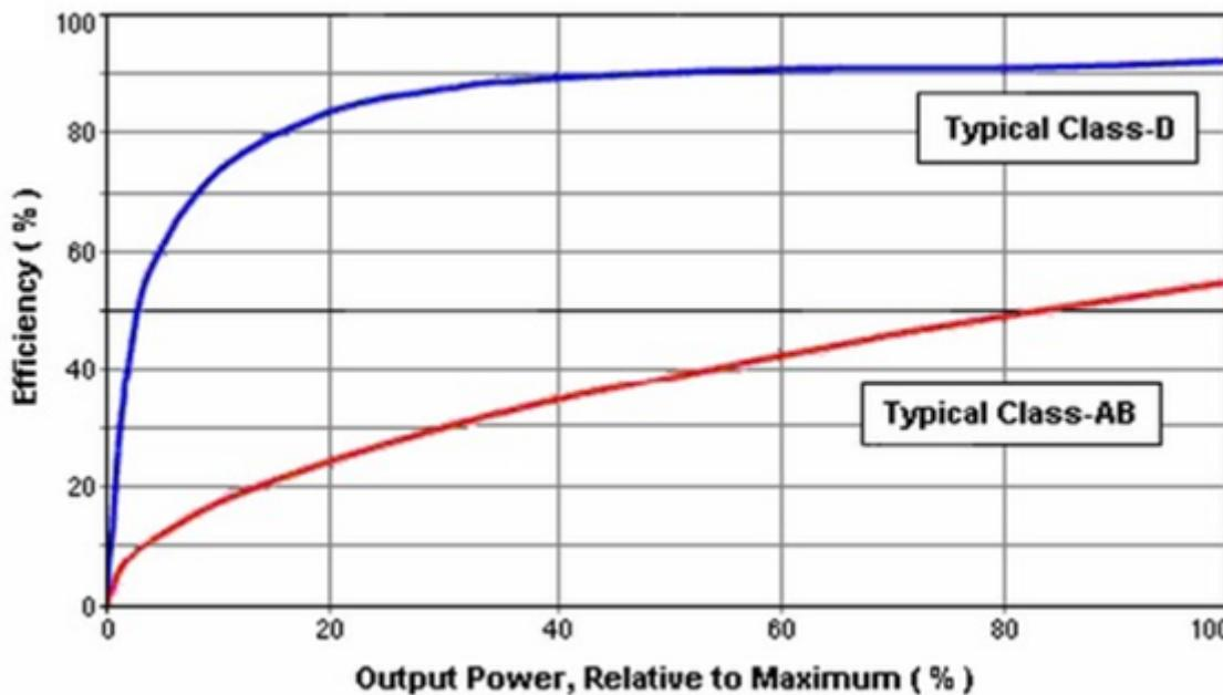
**Figure 2. Class-AB vs. Class-D Efficiency (Image Courtesy of <http://www.audioholics.com>)**
