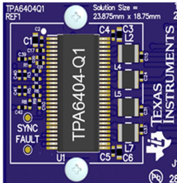
**Figure 5. Four-channel Class-D Amplifier Solution Size**
