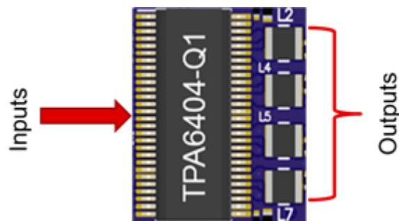
Figure 4. Flow-through Design of the TPA6404-Q1
