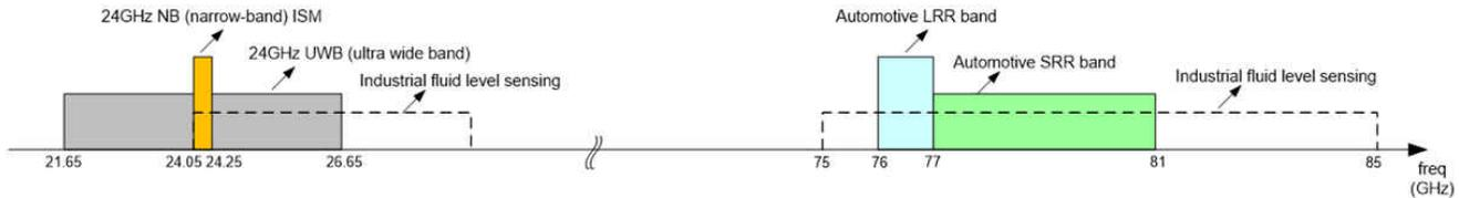
**Figure 2. Available Automotive Radar Bands**
