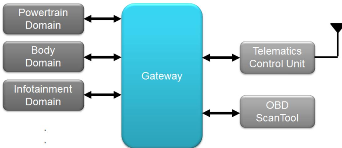
Figure 1. A Typical Vehicle Network Configuration Showing the Gateway
