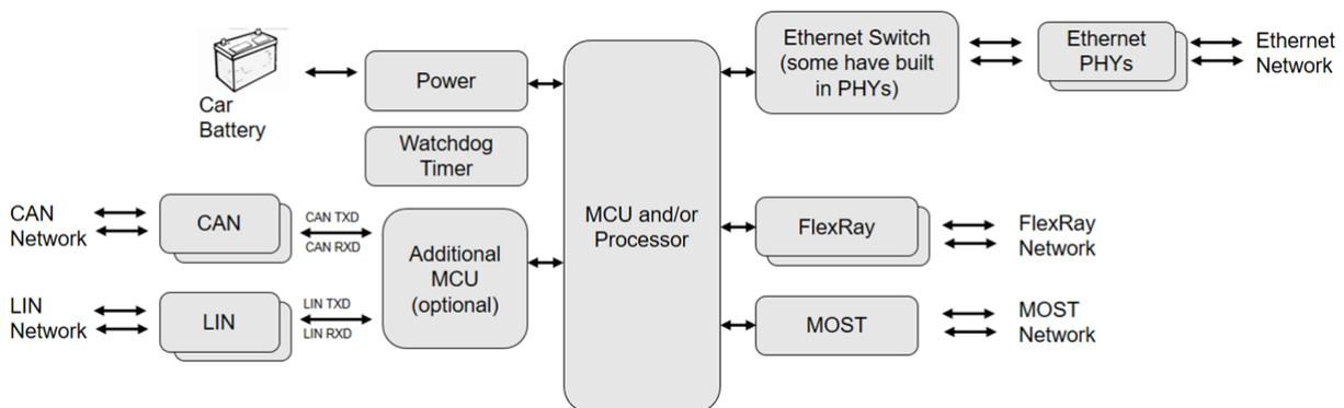
Figure 2. Automotive Gateway Block Diagram
