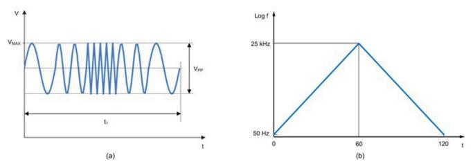
Figure 1. An ISO 16750-2 Superimposed Alternating Voltage Test (a); a Log Frequency Sweep Profile from 50Hz to 25kHz over a Two-minute Sweep Duration (b)
