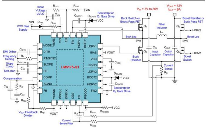
Figure 2. Four-switch Synchronous Buck-boost Solution with a Wide VIN Range of 3V to 36V
