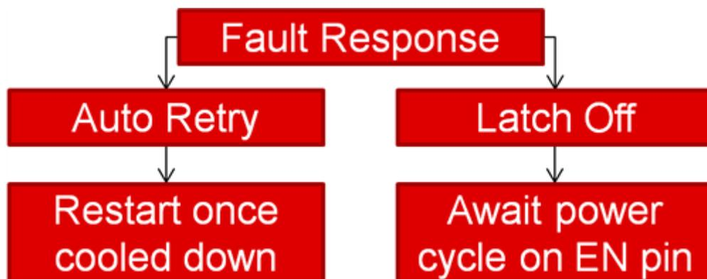
Figure 1. eFuse Fault-response Options (Auto Retry and Latch off)
