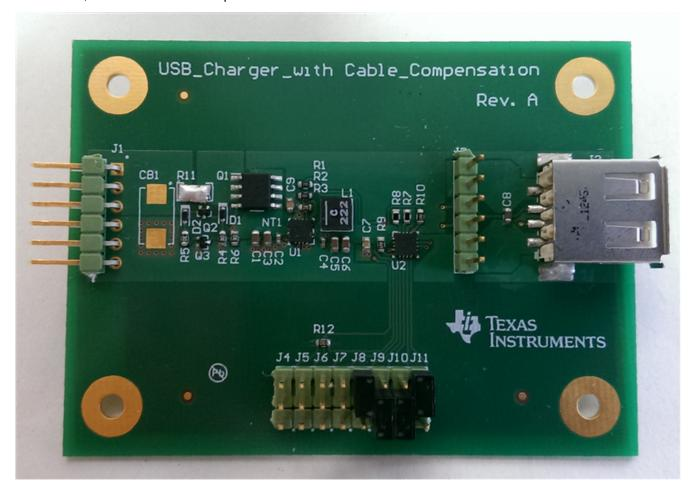
Figure 1. PMP9765 Demonstrates a Complete USB Port Power Solution with Overvoltage Protection and Cable-drop Compensation
