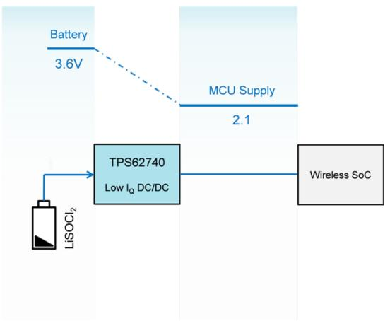
Figure 1. Low  $I_Q$  Power Solution Block Diagram
